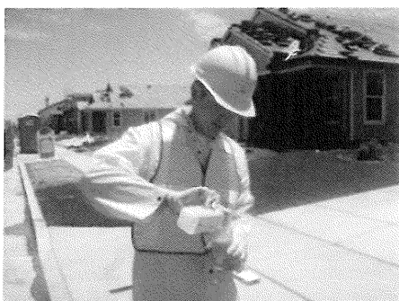
Figure D-5 Transferring sample to field meter sample container
